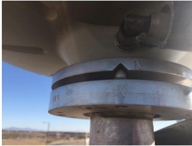
Antenna screwed onto SCIGN mount and oriented to true north.
