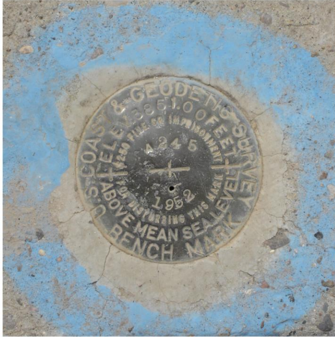
First-order benchmark A-245 on drainage structure headwall across from Mission Inn Best Western - Las Cruces, NM, April 2005.
