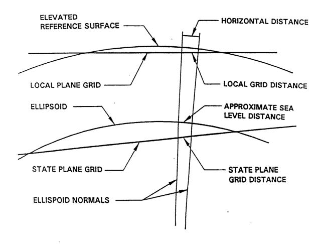
In some cases the difference (distortion) between horizontal ground distance and state plane grid distance is larger than acceptable. An elevated reference surface projection can be used to reduce the distance distortion.
