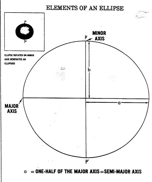
b = ONE-HALF OF THE MINOR AXIS = SEMI-MINOR AXIS
