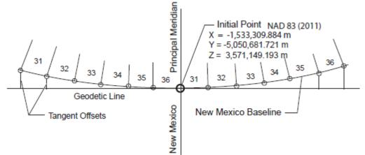
The diagram above presumes that the geodetic line is straight and that the parallel of latitude is curved. The tangent off-sets are the distances between the two lines.
